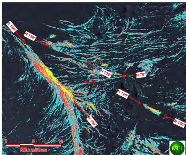
The SAGOM shows a main conductive fracture N160° that reveals deeper aquifers discharging. These aquifers were confirmed by seismic data. A shallow well through these conductive fractures will access freshwater almost from the surface, but drilling deeper should provide access to huge quantities of clean fresh water, in a more sustainable way.
