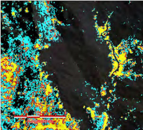
**Figure 1.10.** Example of SAGOM representation of conductive and non-conductive fractures. Conductive, or water-bearing fractures are assigned in yellow lines, while non-conductive or dry fractures are in blue. RTI, 2013.
